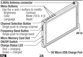
**CAUTION:** Do not power the monitor on without the antenna attached. Doing so will damage the video transmitter and receiver amplifiers. Amplifier damage is not covered by warranty.
