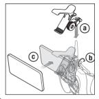
Insert a micro memory card (not included) in the slot on the side of the video monitor. Press the card in until it locks. To remove the card, press in slightly and release until the card is released.
